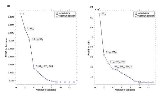
Figure 7. The optimum combination of independent variables to include in a MLR equation to calculate the dependant variable, i.e. BVOC concentrations. The root mean square error (RMSE) difference between the calculated and measured concentrations indicated that the inclusion of (a) 9 parameters for isoprene, (b) 10 parameters for MBO, (c) 7 parameters for MT, and (d) 12 parameters for SQT in the MLR solution was the optimum.
