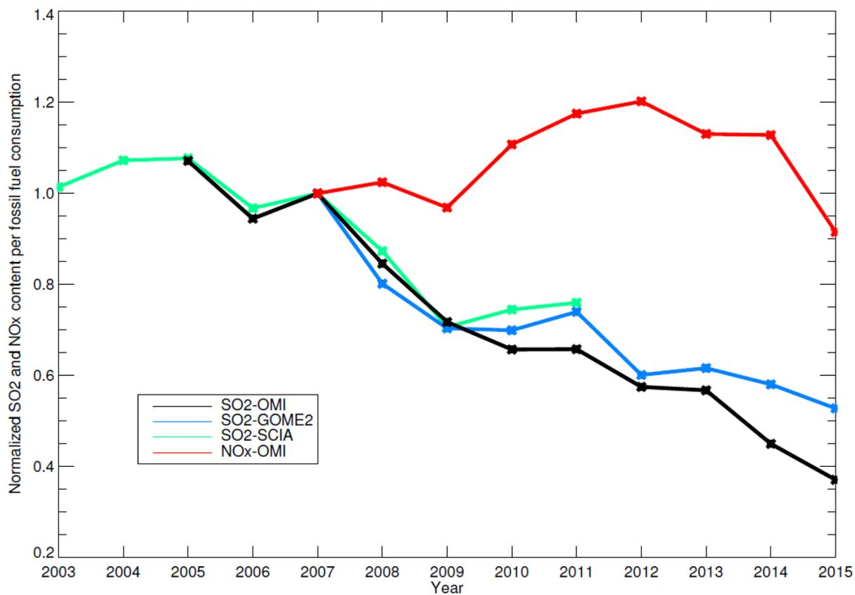
5 **Figure 6: Time series of the ratio of the mean SO<sub>2</sub> columns and the fossil fuel consumption in China based on observations of OMI (black), SCIAMACHY (green), and GOME-2 (blue). The ratios of the annual NO<sub>x</sub> emissions and the fossil fuel consumption is based on observations of OMI (red). All time series are normalized to the year 2007.**
