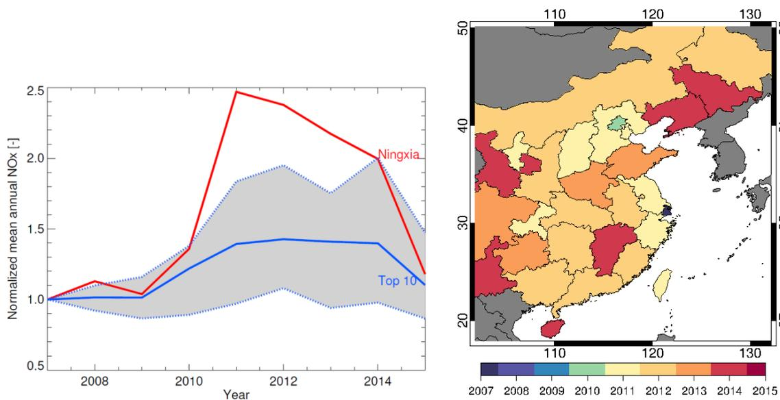
**Figure 4:** (a) Shown are the annual total NO<sub>x</sub> emission estimates for the last 9 years for East China. Emissions are derived with DECSO V4 using OMI observations. (b) Peak year of the NO<sub>x</sub> emissions per province.
