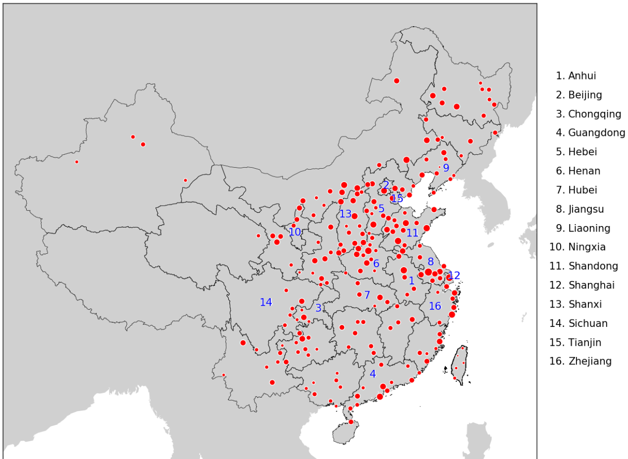
Figure 1: Location of power plants in China according to REAS v.2 (Kurokawa et al., 2013). The size of each dot indicates the emission of the power plants (Power plants in close proximity are combined in a single dot). In addition, a list is given of the provinces mentioned in this study.
