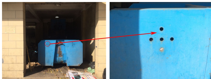
Figure 2. Field photos of a solid waste container in the solid waste transfer station we used for source sampling at Fudan University. Before sampling, an Ogawa passive sampler for \text{NH}_3 is attached on a plastic strip (1.5 m in length). The sampler is fitted into the container through the holes (shown on the right panel).
