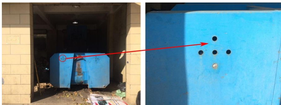
Figure 2. Field photos of a solid waste container in the solid waste transfer station we used for source sampling at Fudan University. Before sampling, an Ogawa passive sampler for \text{NH}_3 is attached on a plastic strip (1.5 m in length). The sampler is fitted into the container through the holes (shown on the right panel).
