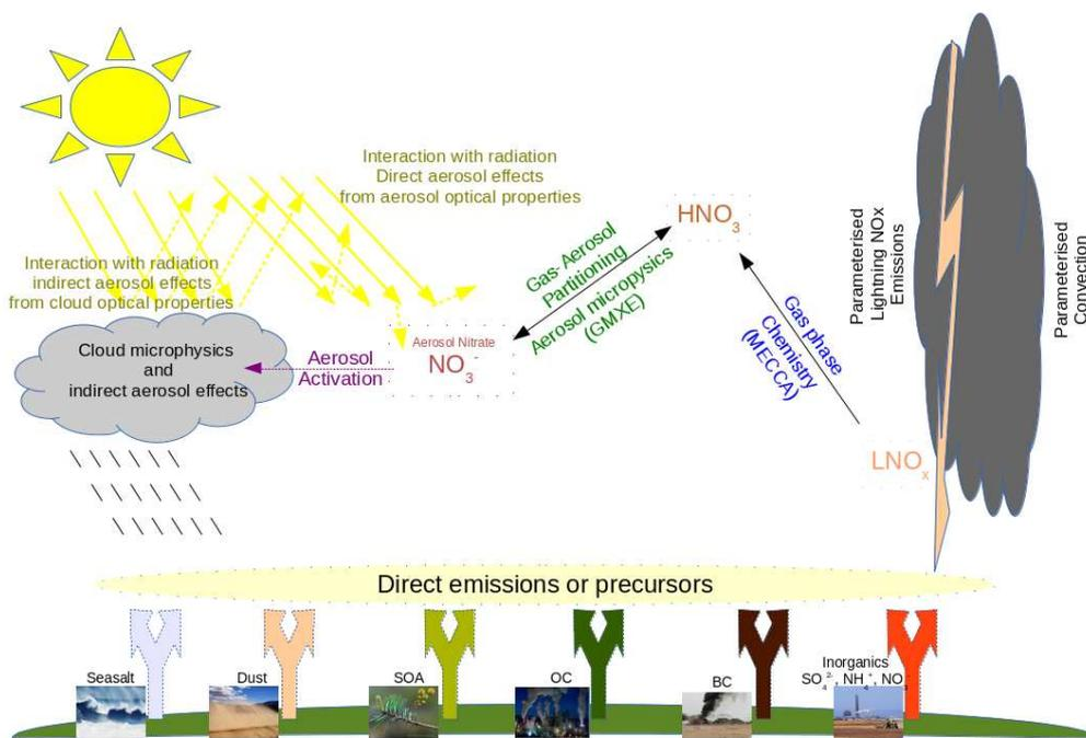
**Figure 1.** Sketch of the simulated processes from the emission of  $\text{NO}_x$  molecules by lightning over gas phase conversion to  $\text{HNO}_3$ , gas aerosol partitioning to particulate  $\text{NO}_3^-$  and implications for the direct and indirect aerosol effects.
