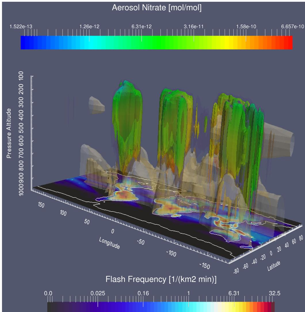
**Figure 2.** 3D visualisation of LNO<sub>x</sub> emissions (coloured isosurface of  $1 \cdot 10^{-16}$  kg/(m<sup>3</sup>s) and darker shaded isosurface of  $3 \cdot 10^{-16}$  kg/(m<sup>3</sup>s)) and the total aerosol nitrate mixing ratios (grey-gray isosurface of 0.1 ppb<sub>v</sub>). Additionally, the mean flash rate in 1/s.(km<sup>2</sup> min) is depicted by the 2D slice at the bottom. Note the logarithmic scaling of both colour bars.
