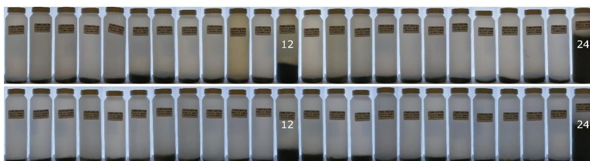
Figure 2: Sediment-trap bottles of the upper (1200 m) and lower (3500 m) traps at station M4 (12°N, 49° W).
