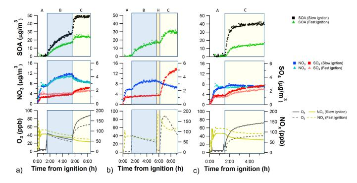
Figure 2: SOA mass and selected trace gas concentrations in a smog chamber for experiments (a) 1B and 2B, (b) 3B, and (c) 4B and 5B. Stabilization (40 min) followed by filling the chamber (35 min) is marked as A, dark aging as B, UV aging as C, and HONO addition as H. NO<sub>3</sub>/5 and O<sub>3</sub>/7 after the HONO addition is shown in Fig 2b.
