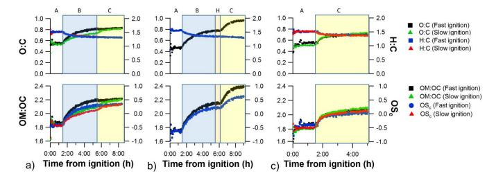
Figure 3: Effect of aging on OA elemental composition for experiments (a) 1B and 2B, (b) 3B and (c) 4B and 5B.
