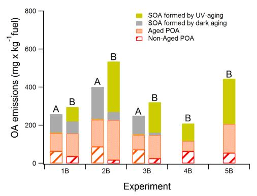
Figure 6: Aged and non-aged POA emission together with SOA at the end of dark (A) and UV aging (B) periods based on PMF calculations (Exp. 1B-5B).
