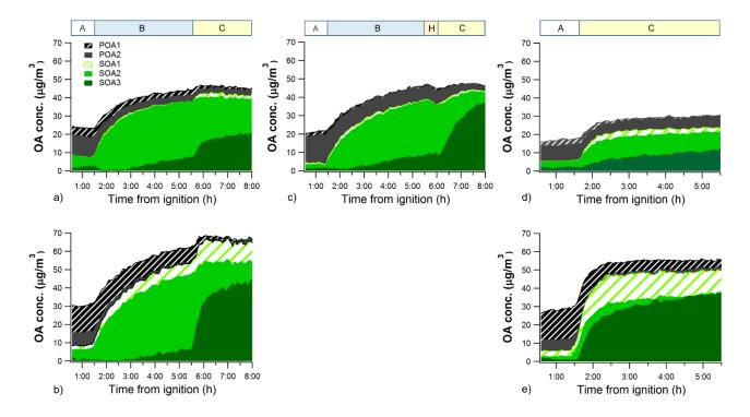
Figure 5: Evolution of OA during aging based on PMF calculations: (a) Exp. 1B, (b) Exp. 2B, (c) Exp. 3B, (d) Exp. 4B, and (e) Exp. 5B. The stabilization phase is marked as A, dark aging as B, UV aging as C, and the HONO addition as H in the upper panel.
