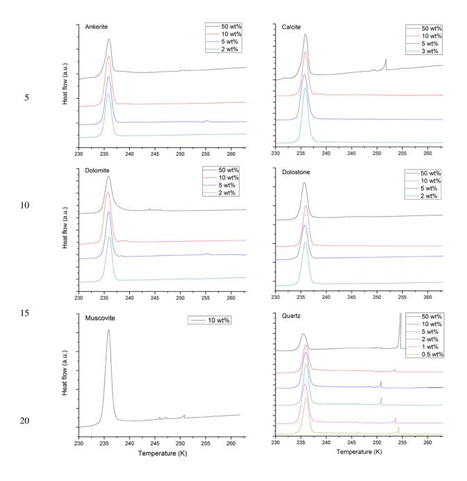
Figure 5a. DSC thermograms of frequently found minerals: ankerite, calcite, dolomite, dolostone, muscovite and quartz. Suspension concentrations are given in the legend.
