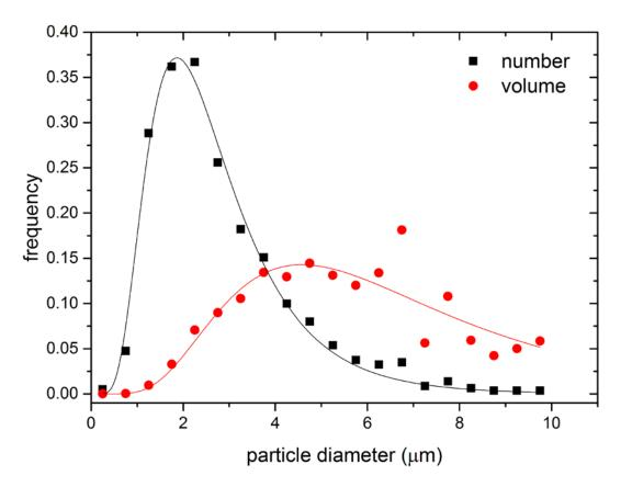
**Figure 1.** Normalized lognormal size distribution of emulsion droplets. Data points represent bin widths of 0.5 μm. The parameters for the lognormal number distribution are  $d_m = 2.41 \pm 0.04$  μm and  $w = 0.507 \pm 0.014$  and for the volume distribution  $d_m = 6.1 \pm 0.4$  μm and  $w = 0.53 \pm 0.05$ .
