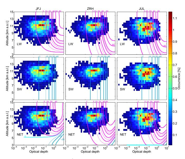
**Figure 8.** Cloud Radiative Forcing (CRF) in  $Wm^{-2}$  for the different sites. Magenta/cyan/blue isolines: positive/zero/negative values in  $Wm^{-2}$  from the CRF model (Corti and Peter, 2009). Color coding: Occurrence frequency of cirrus clouds as function of optical depth and cloud top altitude. First row: CRF<sub>LW</sub>. Second row: CRF<sub>SW</sub>. Third row: CRF<sub>NET</sub>.
