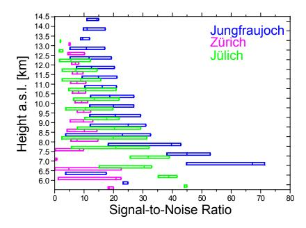
**Figure 5.** Vertical distribution of the signal-to-noise ratio of the detected cirrus clouds for Jungfraujoch, Jülich, and Zürich. The center line of each box plot represents the median. The left and right limits of the box plots mark the 25% and 75% percentiles, respectively.
