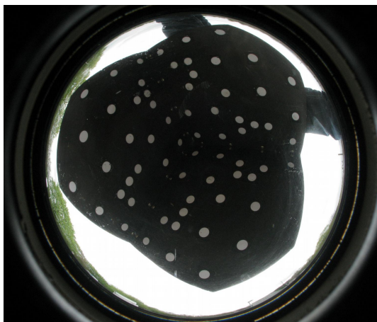
Figure 6. Camera calibration with cube: the pattern on the inside of the cube defines a set of 3D points with respect to the cube coordinate system and can be used as reference data to solve for the fisheye projection parameters.
