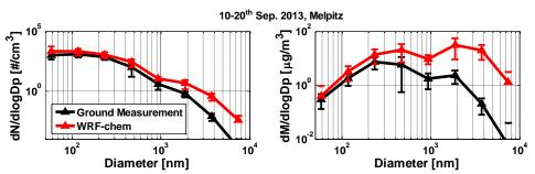
**Figure 3.** Comparison of Particle Number Size Distribution (PNSD, left) and Particle Mass Size Distribution (PMSD, right) between F-CASE simulation and Melpitz measurements. Model results indicated by the red lines and measurements by the black lines. The result is averaged in the period September 10-20, 2013, the error bar indicate the upper and lower limits.
