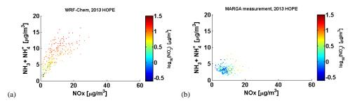
**Figure 7.** Relationship between nitrate, total ammonia and NOx during September 10-20, 2013 at Melpitz. The color indicates the nitrate mass concentration in logarithmic scale. (a) WRF-Chem model results; (b) MARGA measurement results.
