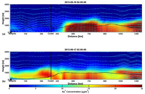
**Figure 6.** WRF-Chem result of the sea salt (Na<sup>+</sup>) concentration on the vertical cross section, which is shown by the black dash line in Figure 1. The locations of Melpitz and coast are marked by black five-point star and black solid line. The light blue arrows indicate the wind field, and the black dash line indicates the planetary boundary layer (PBL) height. (a) 2013-09-16, 04:00 LT; (b) 2013-09-17, 02:00 LT.
