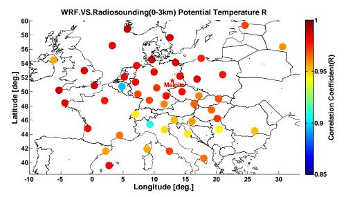
**Figure 2.** Correlation coefficient (R) map of the potential temperature under 3 km between WRF-Chem model and radio-sounding measurements. Melpitz is marked as red star.
