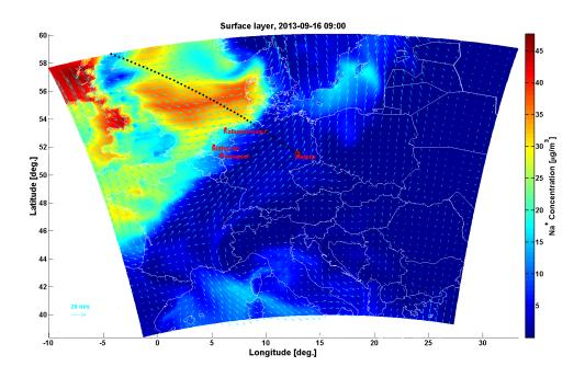
**Figure 1.** The horizontal distribution of surface Na<sup>+</sup> mass concentration in domain 02 at 2013-09-16, 09:00 LT. The light blue arrows indicate the wind field. The locations of 4 EMEP stations (Melpitz, Bilthoven, Kollumerwaard and Vredepeel) are marked. The vertical cross section of dash black line is shown in Figure 5.
