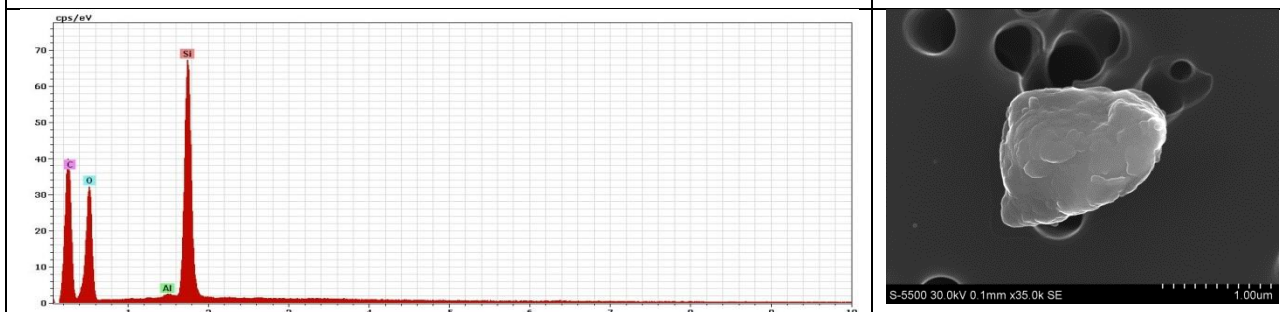
Sample S3011: USA, Colorado, Ft Carson. Rounded particle of quartz (Si) with clay (Al, Si) coating
