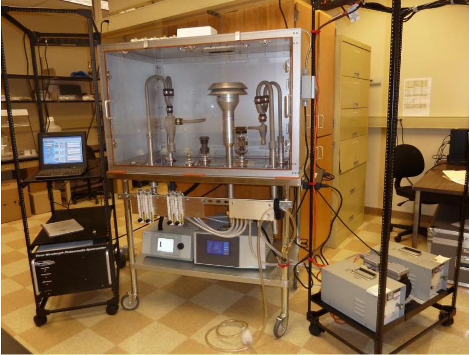
5 Figure 2: Integrated dust entrainment facility: Three-wavelength photoacoustic instrument (DMT PASS-3) on rack to the left, re-suspension chamber on trolley in the center, with a particle size analyzer and beta-attenuation gauge installed below the chamber, and an array of vacuum pumps on rack to the right.
