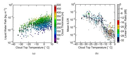
**Figure 10.** (a) LWP of all clouds under study is shown in dependence of temperature and mean cloud top thickness. (b) The ratio between IWC<sub>CB</sub> and mean LWC is calculated for each cloud-profile and average for each cloud case.
