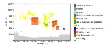
**Figure 4.** Example of automated detection of mixed-phase cloud layers on the basis of the Cloudnet target classification scheme for 2 October 2012. Blue squares mark liquid-only layers and red squares mark mixed-phase layers. The colors are only for a very basic visualization of the layer detection. The decision between mixed-phase and liquid clouds in the following analysis is more complex and described in the text.
