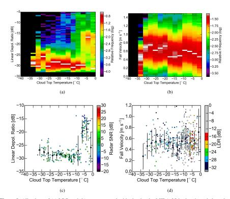
**Figure 9.** All values of (a) LDR and (b)  $v_{CB}$  measured with cloud radar MIRA-35 in the virgae below cloud layers over Leipzig. Averaged values for the indivdual cloud cases are depicted in (c) and (d), respectively. Maximum values in each column are marked with white bars.
