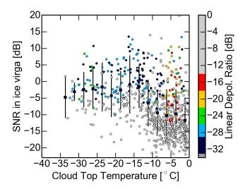
Figure 6. The 90% percentile of cloud-radar SNR is shown for each cloud case together with mean detected LDR.
