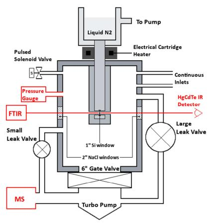
Figure 1: Schematic drawing of the reactor used in this work. The diagnostic tools are highlighted in red and important parameters are listed in Table 1 and Table 2. The ice film is
