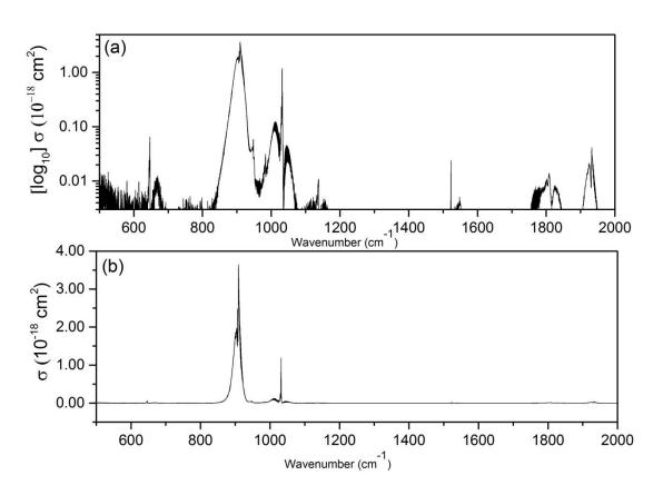
Figure 1. Infrared absorption spectrum of  $NF_3$  at 295±2 K on a logarithmic (a) and linear (b) scale. The logarithmic 5 plot highlights the minor bands.
