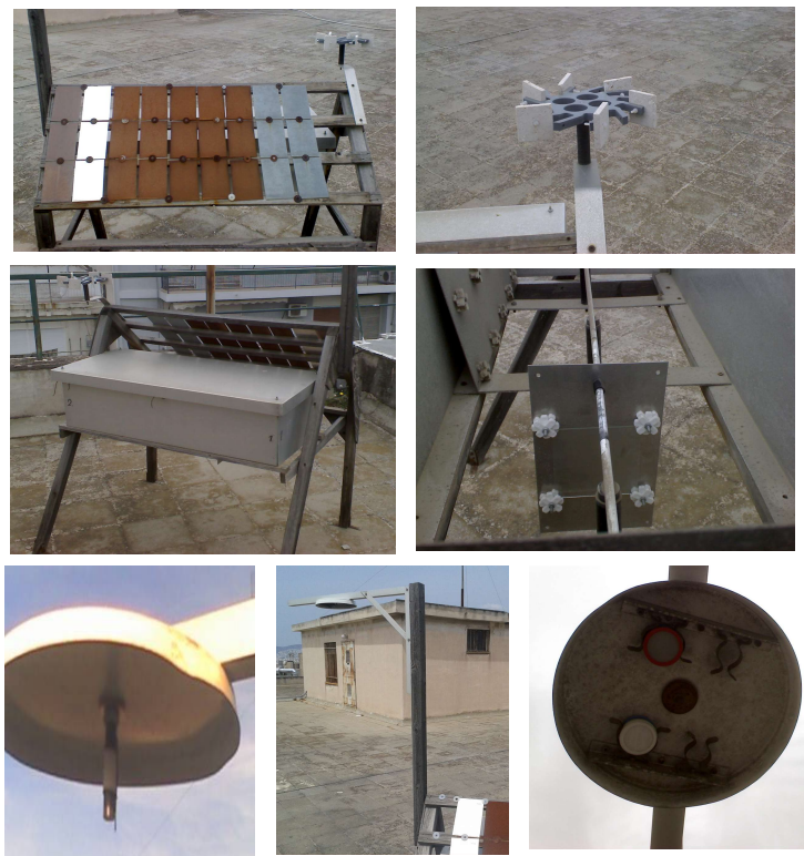
5 Figure 1: The exposure site in the Athens centre (Greece). The top panel shows the carousel (on the right) and the main rack (on the left) with the material specimens, which was installed in Athens and consisted of an inclined plane and an aluminium box with open bottom (middle panel). The middle panel shows aluminium box (on the left) and the glass specimens in the aluminium box (on the right). The bottom panel shows the diffusive passive samplers for the surface air-pollutants measurements and the passive particle collector under the rain shield.
