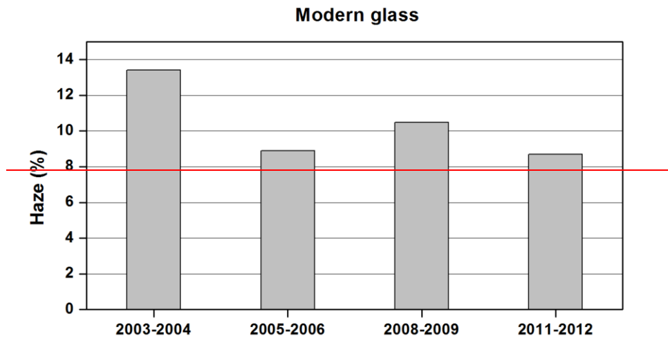
Figure 10: Haze (%) for modern glass exposed for the periods 2003-2004, 2005-2006, 2008-2009 and 2011-2012.
