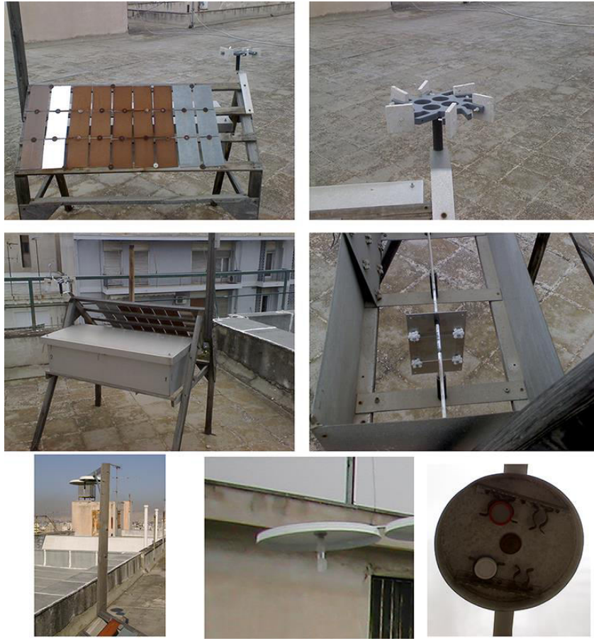
Figure 1: The exposure site in the Athens centre (Greece). The top panel shows the carousel (on the right) and the main rack (on the left) with the material specimens, which was installed in Athens and consisted of an inclined plane and an aluminium box with open bottom (middle panel). The middle panel shows aluminium box (on the left) and the glass specimens in the aluminium box (on the right). The bottom panel shows the diffusive passive samplers for the surface air-pollutants measurements and the passive particle collector under the rain shield.
