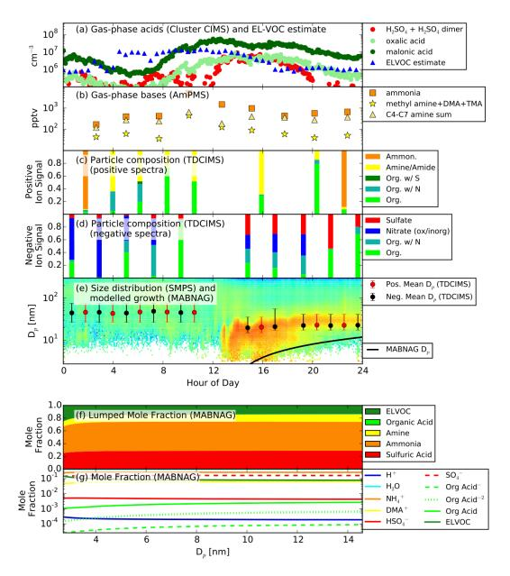
Figure 4: Measurements and MABNAG predictions for the base-case simulation, MAL/10ox/DMA\_L, for May 11, 2013. (a) Gas-phase acids and ELVOC estimate. (b) Gas phase bases. (c)-(d) Particle-phase data. (e) Size distribution from the three merged SMPSs with the modeled growth rate (black line). Overlaid is the mean
