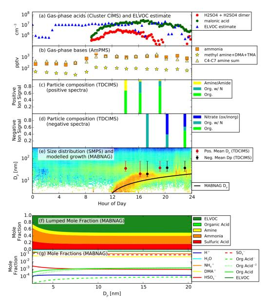
Figure 2: Measurements and MABNAG predictions for the base-case simulation, MAL/100x/DMA\_L, for April 19, 2013. (a) Gas-phase acids and ELVOC estimate. Oxalic acid was not measured for this day; the cluster CIMS was not operational before 9:00 CDT for this day. (b) Gas phase bases. (c)-(d) Particle-phase data. The TDCIMS was not
