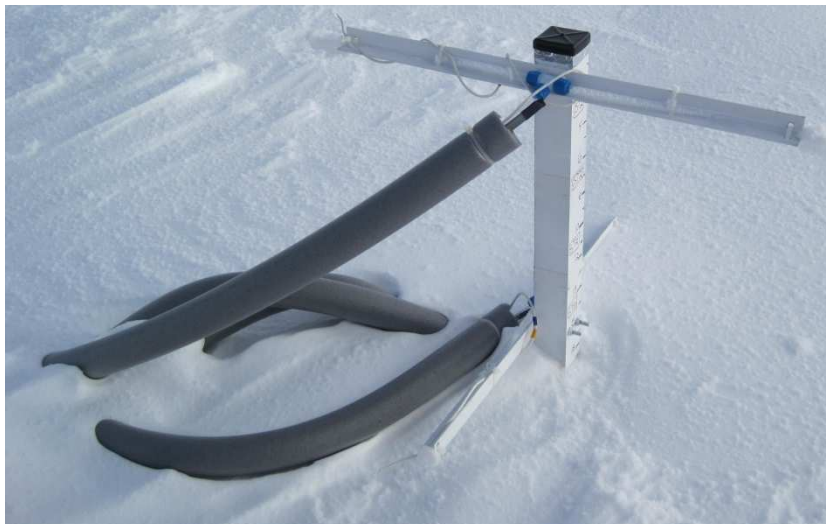
Figure 2: Photographs showing a) the meteorological tower with the three gas inlets (red arrows) at 1070 cm, 210 cm and 25 cm above the snow surface (photo credit: B. Jourdain), and b) one of the snow towers with the two sampling inlets above the snowpack at 50 and 10 cm (photo credit: D. Helmig).
