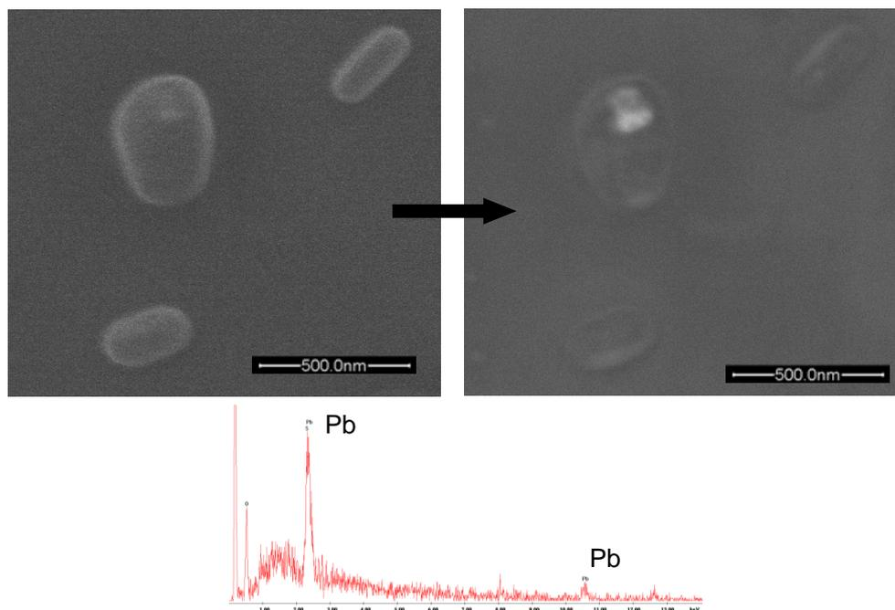
**Figure 5: Left: Three secondary particles containing different amounts of sulphates/nitrates/organics at the beginning of electron microscopic investigation. Right: Under electron bombardment the material is evaporizing after a few seconds exhibiting a lead rich inclusion.**
