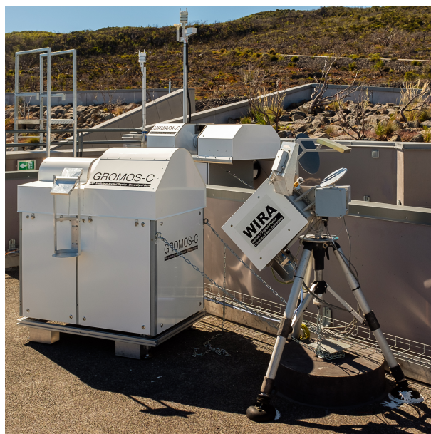
Figure 1. The ozone radiometer GROMOS-C at the Maïdo observatory, in La Réunion Island, together with the wind radiometer WIRA and the water vapour radiometer MIAWARA-C.
