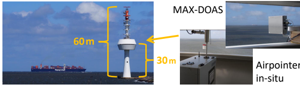
Figure 2. Radar tower Neuwerk with MAX-DOAS and in-situ measurement device
