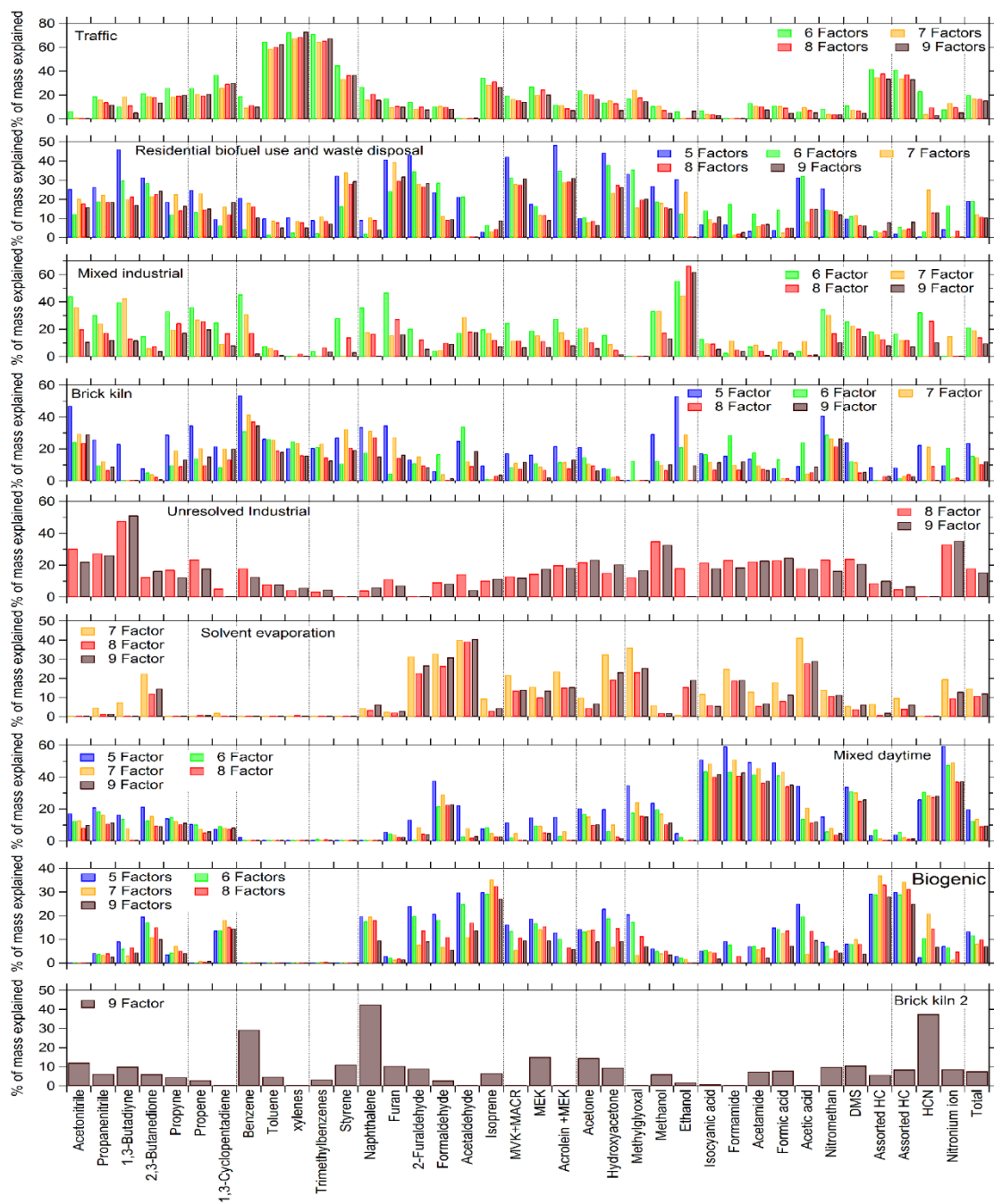
Figure S3b. Evolution of the percentage of the mass of each compound explained by the eight sources identified and the 9 th source which is considered to arise due to splitting of the brick kiln factor from the 5 Factor to the 9 Factor solution.
