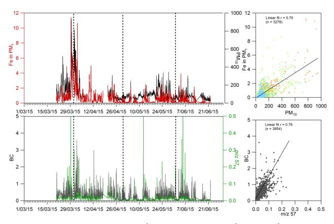
Fig. 4. (Left) Time series of (top) Fe and  $PM_{10}$  concentrations (in  $\mu g$  m<sup>-3</sup>) and (bottom) BC concentration (in  $\mu g$  m<sup>-3</sup>) and m/z 57 (ng m<sup>-3</sup>) 30 min average. (Right) Corresponding scatter plots and their respective linear fits with Fe and  $PM_{10}$  data colored in red for continental, green for sea breeze and blue for marine days and BC and m/z 57 in grey dots.
