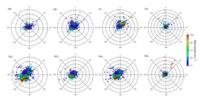
Fig. 8. Pollution rose plots of OM, BC, Chl, Fe, SO<sub>4</sub>, NO<sub>3</sub>, NH<sub>4</sub> and total PM<sub>1</sub> for the whole IOP-1, with concentrations ( $\mu g \ m^{-3}$ ) as radius and colored by wind speed (measurements inferior to 1 m s<sup>-1</sup> in grey).
