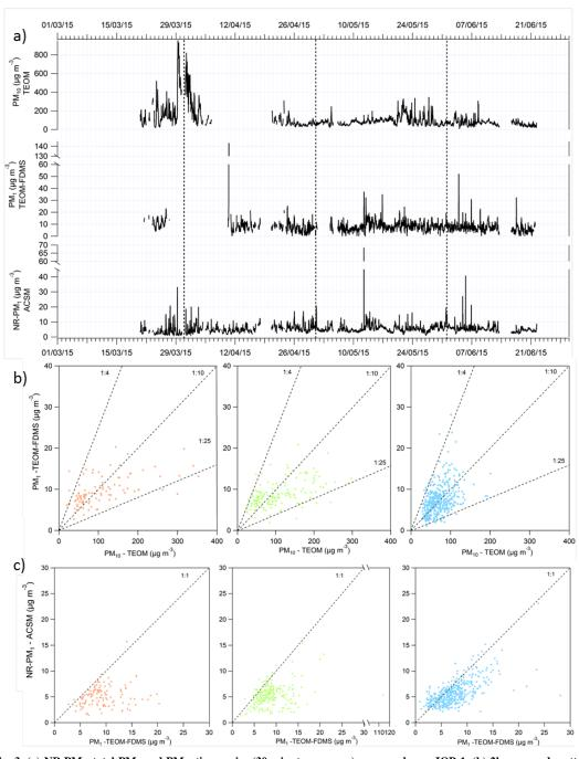
Fig. 3. (a) NR-PM<sub>1</sub>, total PM<sub>1</sub> and PM<sub>10</sub> time series (30-minute averages) measured over IOP-1, (b) 2h averaged scatter plots of total PM<sub>1</sub> vs PM<sub>10</sub> and (c) NR-PM<sub>1</sub> vs PM<sub>1</sub> for (left) continental, (middle) sea breeze and (right) marine days (dotted lines are visual markers representing ratios between the different variables).
