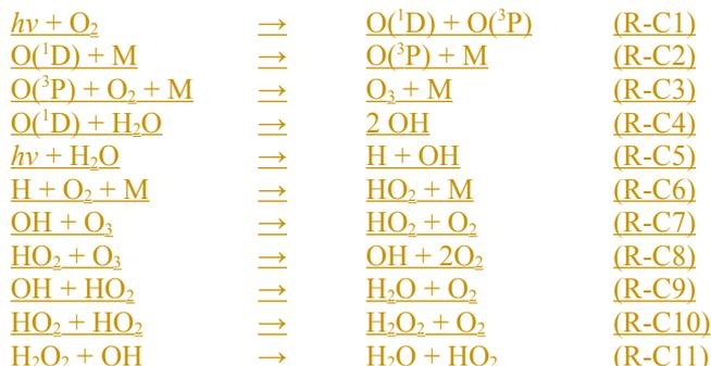
The humidified air flow is exposed to the 172 nm radiation for 50 ms and is then within 30 ms transferred to the mixing zone with the sample flow. The oxidant species produced are OH, HO<sub>2</sub>, O<sub>3</sub> and H<sub>2</sub>O<sub>2</sub>. The final OH concentration entering the mixing zone depends on the residence time in the lamp and in the transfer region.
