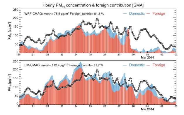
Figure 8: Time series of surface PM10 concentration over the SMA from observations and models during the period from 20 February, 2014 to 3 March, 2014. Contributions from domestic and foreign emissions are shaded with blue and red, respectively.
