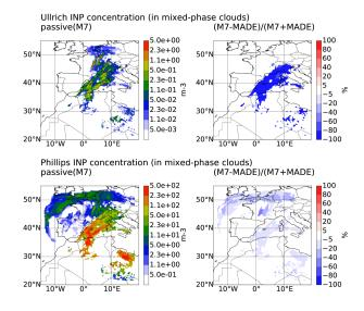
**Figure 12. Mixed-phase INP** concentrations derived from aerosol compositions predicted by M7 (left) and MADE (relative-difference plots on the right) using the Ullrich (first row) and Phillips (second row) parameterizations for **passive** simulations. See Figure 3 for plot details. Contours show vertical averages of concentrations in grid boxes that contain both, ice- and liquid-phase, cloud water.
