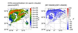
**Figure 10. Liquid-cloud CCN** concentrations derived from aerosol compositions predicted by M7 (left) and MADE (percentage-difference plot on the right) for **passive** simulations. Contours show vertical averages of concentrations in grid boxes that contain liquid-phase but no ice-phase cloud water.
