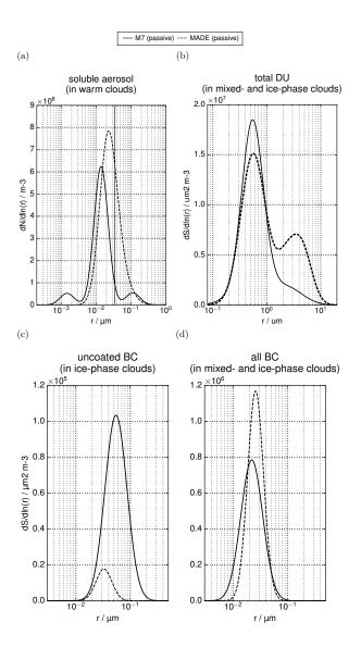
**Figure 11. Size distributions of cloud-active aerosol** for simulation **passive** using MADE and M7. Shown are the CCN-relevant number distribution of soluble aerosol in liquid clouds (a) as well as surface distributions of dust (b) and uncoated (c) and total soot (d) in the cloud regimes where these species serve as INP (Table 2).
