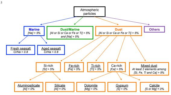
Figure 3. Particle classification (colored text) and identification (underlined text) based on normalized atomic percentages for elements with Z > 10.
