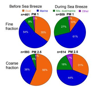
Figure 8. Relative proportions of particle types obtained from CCSEM/EDX analysis of particles collected (left) before the sea breeze and (right) during the sea breeze. Fine and coarse fractions correspond to the aerodynamic cut-off diameters of the cascade
