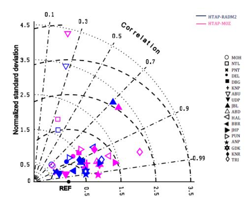
Figure 12. Taylor diagram showing model statistics (r, normalized standard deviation and RMSD) at all sites. The correlation is the cosine of the angle from the horizontal axis, the root mean square difference is the distance from the reference point (REF) and the standard deviation is the distance from the origin.
