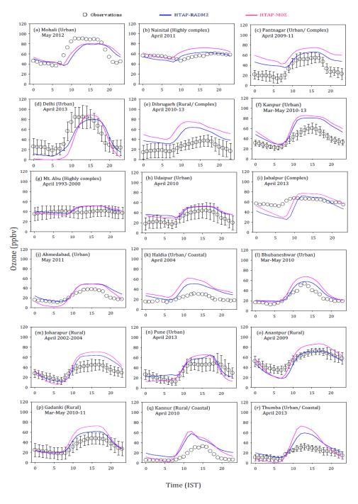
**Figure 11.** Comparison of monthly average diurnal variation of surface ozone simulated using different chemical mechanisms at various observation sites. The observational data is available for the period indicated in the figure whereas all the model simulations are for the year 2013. Error bars represent the temporal standard deviations of the monthly averages. All model simulations are with HTAP inventory.
