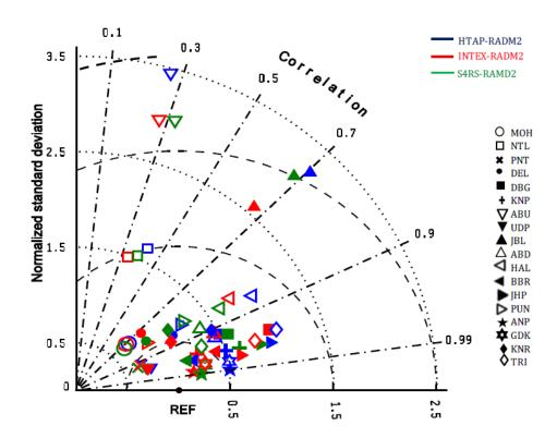
Figure 7. Taylor diagram showing model statistics (r, normalized standard deviation and RMSD) at all sites. The correlation is the cosine of the angle from the horizontal axis, the root mean square difference is the distance from the reference point (REF) and the standard deviation is the distance from the origin.
