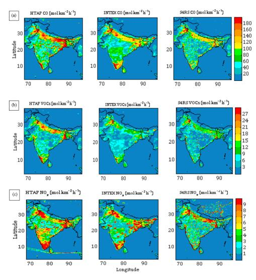
Figure 2. A comparison of (a) CO, (b) NM VOC and (c)  $NO_x$  emissions between the three inventories used (see Section-2.2 for description).
