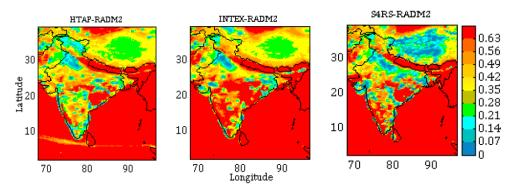
$\textbf{Figure 5. Spatial distribution of net day time surface CH$_2O$ to NO$_y$ ratio in simulations with different inventories for the month April during 0630-1230 IST$
