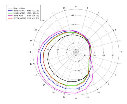
**Figure 14.** Polar plot for monthly mean diurnal variation of surface ozone (in ppbv) from all model simulations and observations each spatially averaged over all sites. The numbers on the outermost circle represent the hour of the day and the radial distance from the centre represents surface ozone mixing ratios in ppbv. The normalized mean bias (NMB in %) values in all the simulations are also provided in the caption box.
