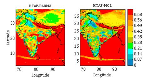
Figure 10. Spatial distribution of net daytime surface  $CH_2O$  to  $NO_y$  ratio in simulations with different chemical mechanisms for the month April during 0630-1230 IST
