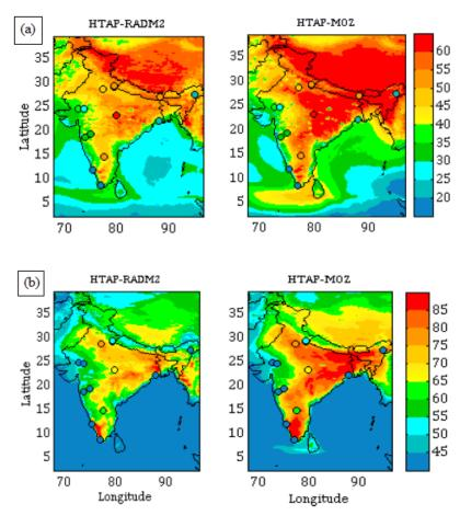
**Figure 8.** Spatial distribution of monthly (April) average surface ozone calculated for (a) 24 h and (b) noontime (1130-1630 IST), comparing the chemical mechanisms (RADM2 and MOZART). The average ozone mixing ratios (ppbv) from observations are also shown for comparison on the same colour scale. Note the difference in colour scales in the top and bottom rows.
