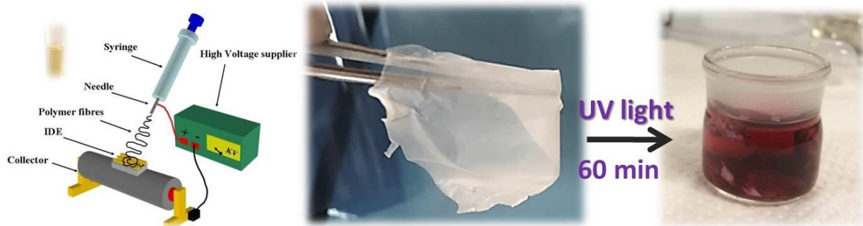
20 Figure 1. Sketch of an electrospinning set-up comprising a syringe and a grounded rotating cylinder collector where the samples take place for their coverage (left); a piece of a nanofibrous fabric of \text{TiO}_2/\text{PVP} removed from the substrate after 1 h of electrospinning deposition (centre); a red-purple aqueous solution of \text{HAuCl}_4/\text{PVP} after UV-light irradiation treatment holding a piece of the nanofibrous fabric of \text{TiO}_2 ( anatase ) obtained after \text{TiO}_2/\text{PVP} annealing (right)
