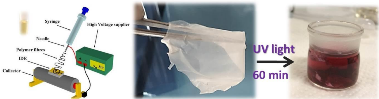
Figure 1. Sketch of an electrospinning set-up comprising a syringe and a grounded rotating cylinder collector where the samples take place for their coverage ( left ); a piece of a nanofibrous fabric of \text{TiO}_2/\text{PVP} removed from the substrate after 1 h of electrospinning deposition ( centre ); a red-purple aqueous solution of \text{HAuCl}_4/\text{PVP} after UV-light irradiation treatment holding a piece of the nanofibrous fabric of \text{TiO}_2 ( anatase ) obtained after \text{TiO}_2/\text{PVP} annealing ( right )
