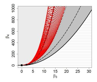
As shown in the figure, the Johnson SB distribution has a wider domain respect to the mixture of two lognormals, indicating that the Johnson SB distribution is more versatile respect to the mixture of two lognormals in representing the OPC data.
