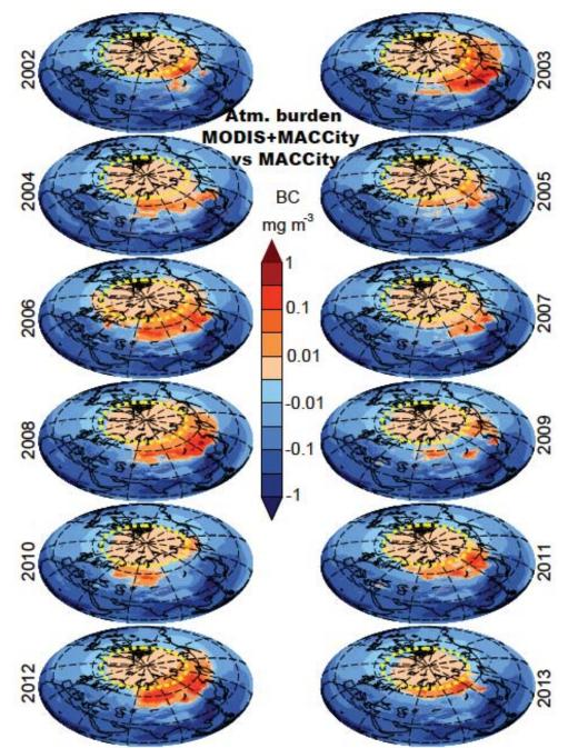
Figure 8. Difference in BC atmospheric burden (mg m<sup>-3</sup>) between our simulation that combines emission inventories (FEI-NE+MACCity) and MACCity. The dashed yellow line represents the limit of the Arctic (~67°N). The BC burden was estimated by averaging all the vertical layers over 365 days for each year from 2002 to 2013.
