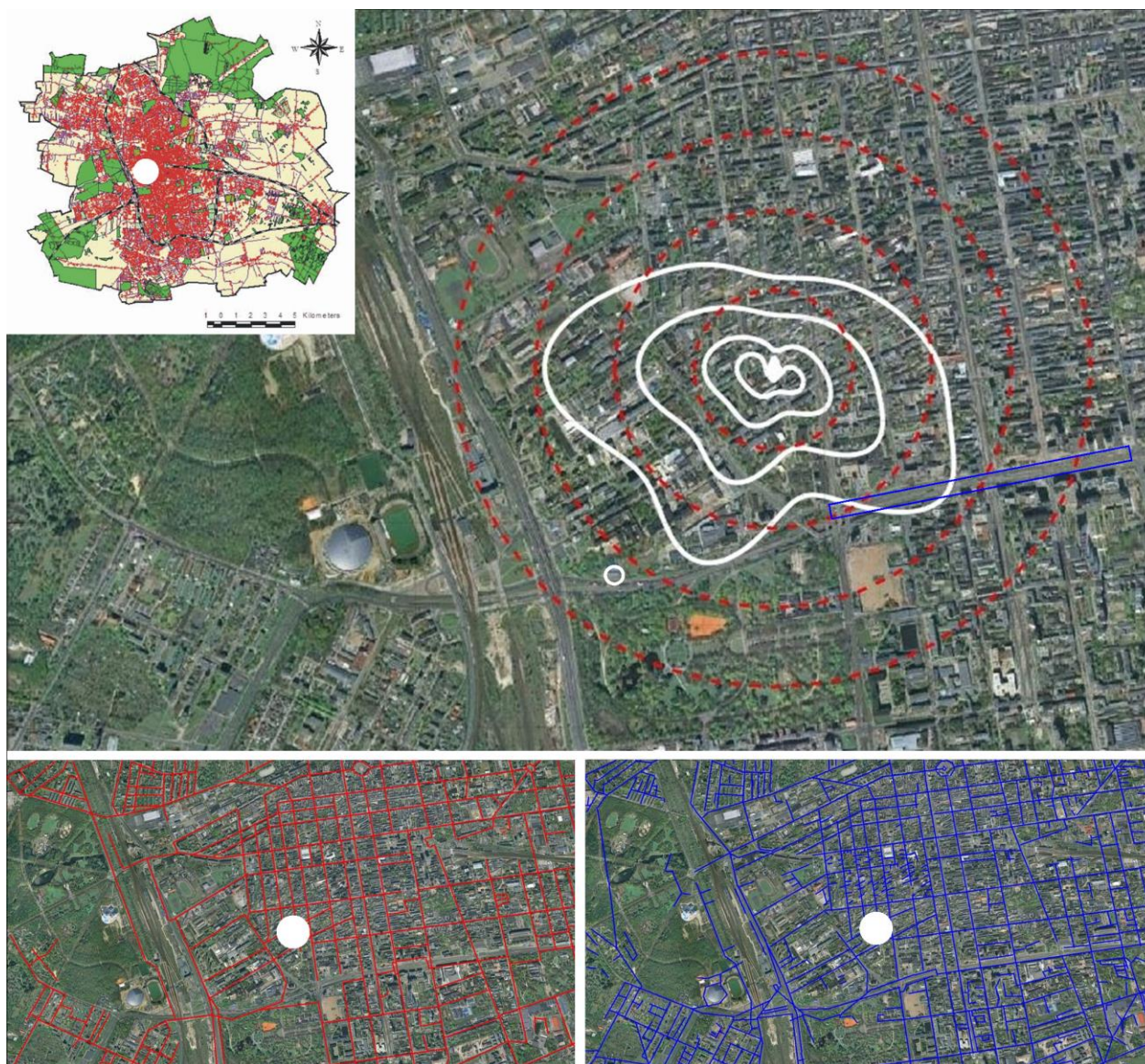
1 2 Figure 1. The western part of the center of Łódź (top). Solid white lines indicate the source 3 area with P = 25, 50, 75 and 90\% , calculated for the turbulent fluxes measured at 10 a.m. to 2 4 p.m. during unstable stratification (all available data from the period July 2013 - August 5 2015). The dashed red lines represent the 250, 500, 750 and 1000 m distance from the 6 measurement point. White circle indicates LPG station and blue rectangle indicates area of 7 road tunnel construction. Bottom figures show spatial distribution of gas network (bottom 8 left) and sewage system (bottom right) in the neighbourhood of the measurement site (white 9 dots). Schemes are based on data from Geodesy Center of Łódź ( www.mapa.lodz.pl ). Photo 10 source: www.google.com
