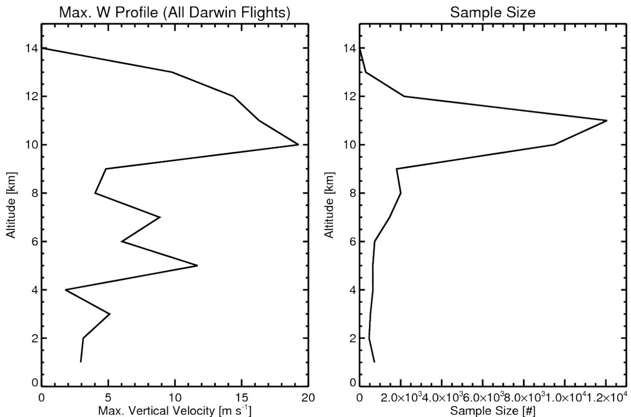
Figure 1. The maximum vertical velocity profile observed by the Falcon-20 aircraft during the HAIC-HIWC Darwin campaign including all flights at 5-second (~750-m) resolution with aircraft roll angles > 5° removed (left). The sample size is shown on the right.
