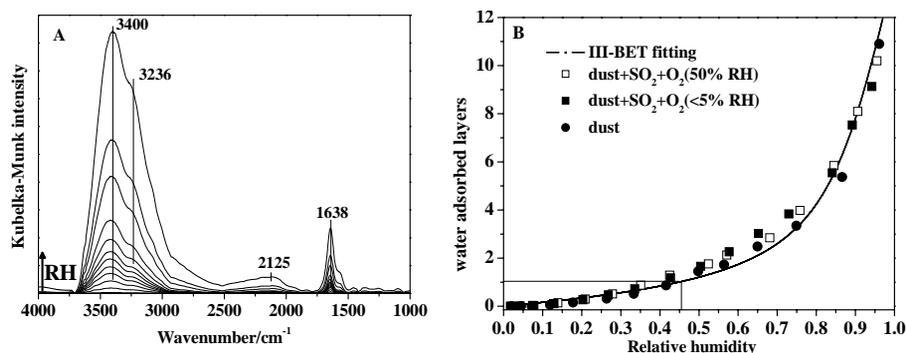
**Fig. 5.** Water uptake on dust particles obtained at 300 K. **(A)** DRIFTS spectra as a function of RH (2.1, 4.5, 7.2, 11.9, 17.8, 26.4, 33.3, 41.6, 49.8, 56.4, 65.0, 74.9, 86.6, 96.1 %RH); **(B)** isotherms of fresh dust, reacted with SO<sub>2</sub> (200 ppm)+O<sub>2</sub>(20%) (<5% RH), and with SO<sub>2</sub> (200 ppm)+O<sub>2</sub> (20%) at RH=50% (50% RH). Integrated region was 2700–3700 cm<sup>-1</sup>.
