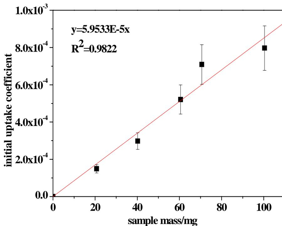
**Fig. 4.** Linear mass dependence of SO<sub>2</sub> observed uptake coefficients on dust particles at 300 K. Conditions of SO<sub>2</sub> flow: 2.0% in N<sub>2</sub> balance.
