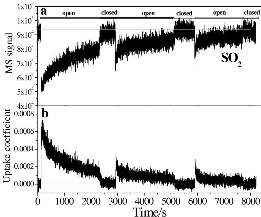
**Fig. 3.** The uptake of SO<sub>2</sub> on 60 mg dust particle at 300 K. **(a)** the temporal concentration profiles for SO<sub>2</sub> ( $m/e=64$ ) in the uptake experiment; **(b)** the observed uptake coefficients. Conditions of SO<sub>2</sub> flow: 2.0% in N<sub>2</sub> balance.
