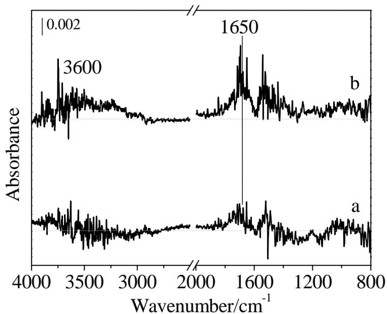
**Fig. 6.** DRIFTS spectra of SO<sub>2</sub> (200 ppm) adsorption on dust particles in air (20% O<sub>2</sub>+N<sub>2</sub>) at 300 K for 2 h in (a) dry condition and (b) humid condition RH=50%.
