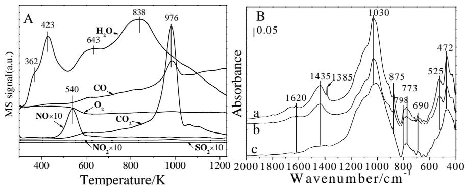
**Fig. 2.** Characterisation of Asian dust storm particles. **(A)** TPD spectra, condition: carrier gas Ar=50 mL/min,  $\beta=20$  K/min,  $m_{\text{sample}}=200$  mg. **(B)** FTIR spectra of (a) fresh sample, heated in air for 12 h at (b) 573 K, and (c) 973 K.
