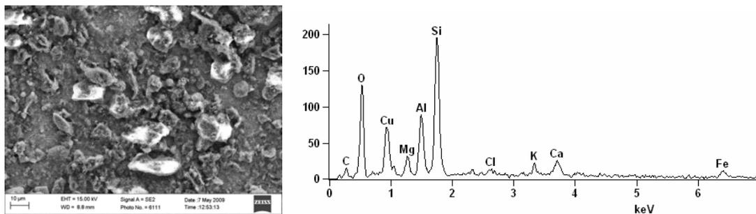
**Fig. 1.** SEM image of dust particle sample (left) and the EDX spectrum (right).
