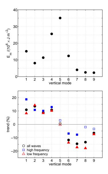
Fig. 3. Top: Vertical spectrum of the mean energy  $(E_m)$  associated with the baroclinic Rossby waves of wave numbers s=1,...,10. Bottom: Linear trends of the November–April mean energy associated with the Rossby waves of wave numbers s=1,...,10, for the first 9 baroclinic modes. The trends are given as percentages of the respective mean energies in the period of 1958–2006. Solid symbols indicate significant trends at the statistical level of 99% (p=0.01).
