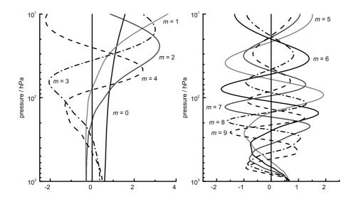
Fig. 1. Vertical structure functions of the barotropic (m=0) and first nine baroclinic modes (m=1,...,9) of the NCEP/NCAR atmosphere. For  $m\geq 2$  one node appears above 10 hPa and it is not represented.
