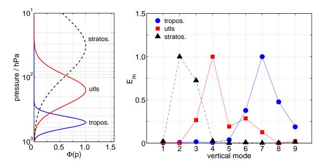
**Fig. A1.** Vertical energy spectra (right) of three idealized geopotential anomalies (left) centered at the middle troposphere, in the UTLS region and in the middle stratosphere. The spectra and the anomalies were normalized to their respective maxima.
