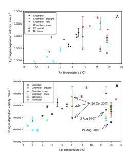
Fig. 2. 'Fig 3 (a) The dependency of measured and modeled hydrogen deposition values (a) to air (b) to soil temperature  $\dots$ '
