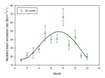
Fig. 3. 'Fig. 5 Two-dimensional model results for 222Rn exhalation rate jRn'
