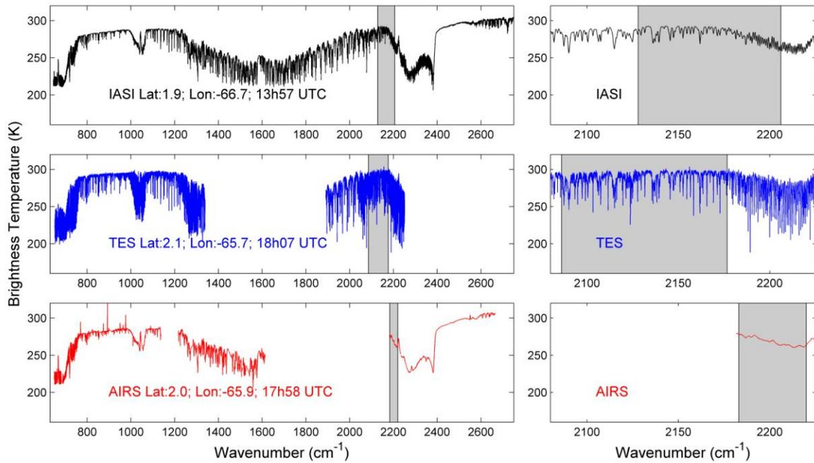
Figure 4. IASI, TES and AIRS radiance spectra (in brightness temperature) around Northern Brazil, on August 1<sup>st</sup>, 2008. The spectral range used for the CO retrieval are highlighted in grey. For the full spectral range covered by each on the left and zoomed for the CO window on the right (IASI [2143 2181.25]; TES [2086.06 2176.66] and AIRS [2181.49 2221.12]).
