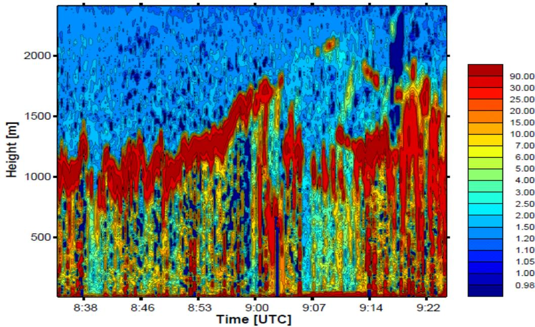
(a) AMALi airborne lidar backscatter profiles on 9 April 2007.
