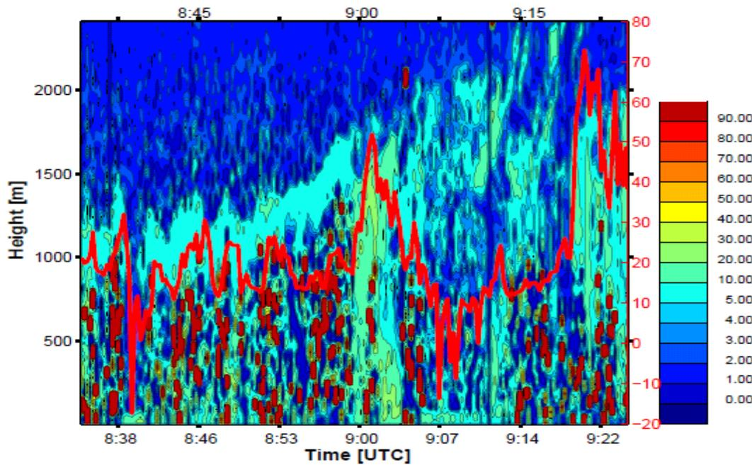
(b) AMALi airborne depolarization profiles on 9 April 2007.
