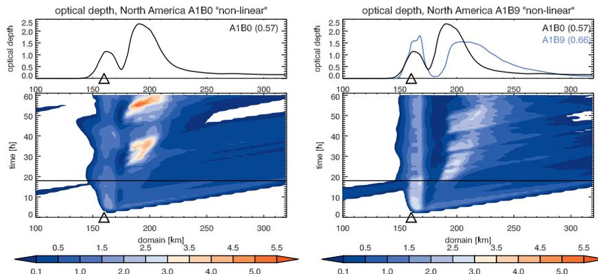
**Fig. 17.** Time development of the optical depth for the A1B0 (left) and A1B9 (right) simulations. The triangle denotes the top of the mountain, and the black line shows the point in time when the flow becomes reasonably stable. The upper panel shows the time averaged optical depth from 3–10 h. In the upper right panel we also show the time averaged optical depth for the A1B0 simulation for a better comparison.
