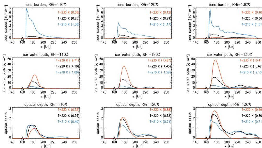
**Fig. 6.** Optical depth, ICNC and IWP after  $t=5$  h for (left) RH=110%, (middle) RH=120% and (right) RH=130%. Different colors indicate different temperatures inside the ISSR. Values in brackets denote the mean values, whereas here all values corresponding to  $\tau > 0.03$  are considered.
