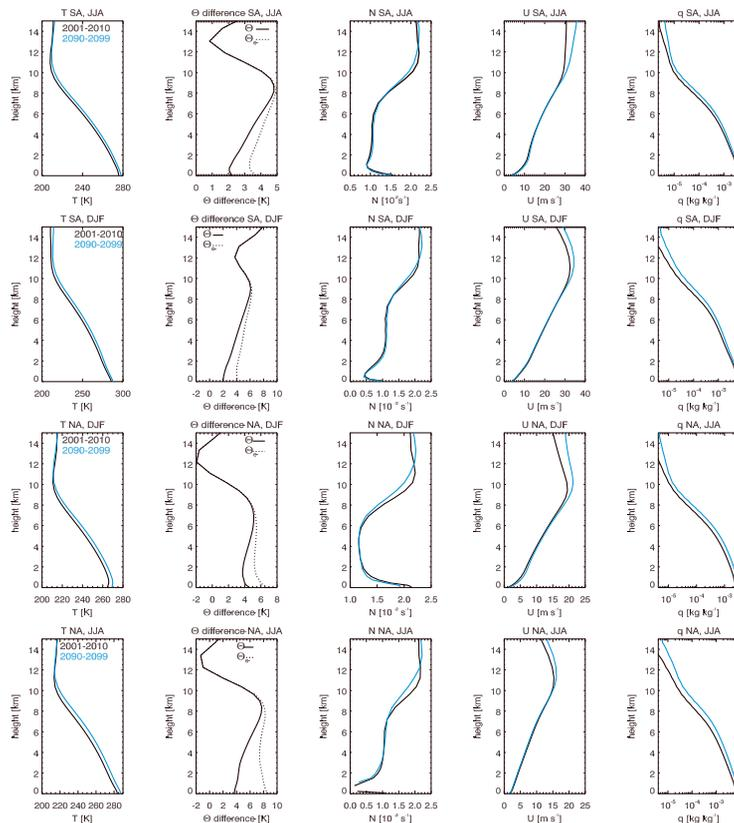
**Fig. 8.** Ten year mean of the initial profiles of temperature  $T$ , difference of potential temperature  $\theta$  and equivalent potential temperature  $\theta_e$  between A1B9 and A1B0, moist Brunt-Väisälä frequency  $N$ , wind speed  $u$  and specific humidity  $q$  for 2001–2010 (black) and 2090–2099 (blue) for the Southern Hemisphere winter and summer month (upper two panels) and Northern Hemisphere winter and summer months (lower two panels).
