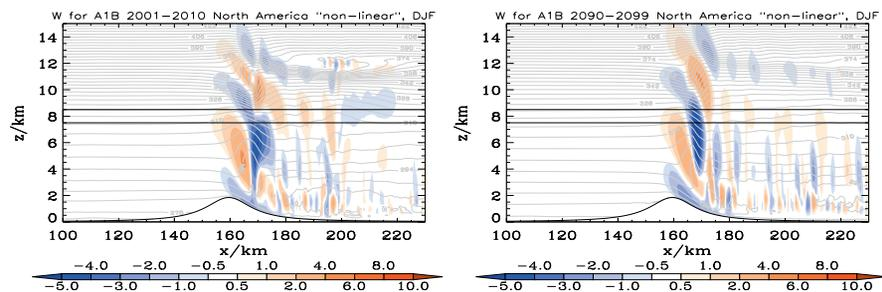
**Fig. 16.** Flow regime for North America after  $t=10$  h for the initial profiles of 2001–2010 (right) and 2090–2099 (left). Grey lines denote the lines of potential temperature, colors indicate the vertical velocity. The black box shows the position of the supersaturated layer.
