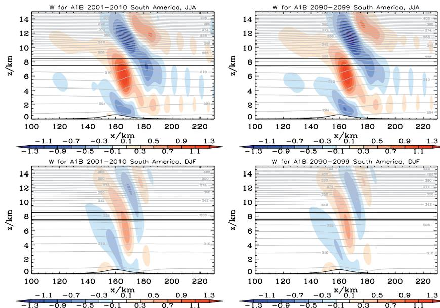
**Fig. 9.** Flow regime for South America after  $t=5$  h for the initial profiles of 2001–2010 (left) and 2090–2099 (right) and for winter (JJA, upper panels) and summer (DJF, lower panels). Grey lines denote the lines of constant potential temperature, colors indicate the vertical velocity. The black box shows the position of the supersaturated layer.
