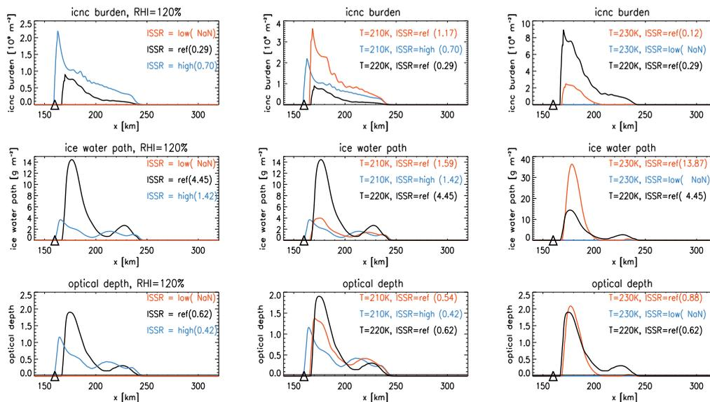
**Fig. 7.** Optical depth, ICNC and IWP after  $t=5$  h for (left) RHi=120% and three different positions of ISSR, (middle) comparison of a decrease in temperature due to a change of the height of the ISSR (blue line) and shift of the initial temperature profile (red line) to  $T=210$  K at RHi=120% and (right) same as in the middle panel but for a temperature increase to  $T=230$  K at RHi=120%. Note that the vertical axis differs in each column.
