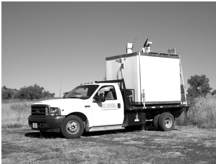
Fig. 1. The University of Iowa mobile vertical lidar (1064 nm 50 Hz 25 mJ/pulse laser, 100 MHz digitizer, 1.5 m spatial and 1 s temporal resolution) during the MILAGRO 2006 campaign.
