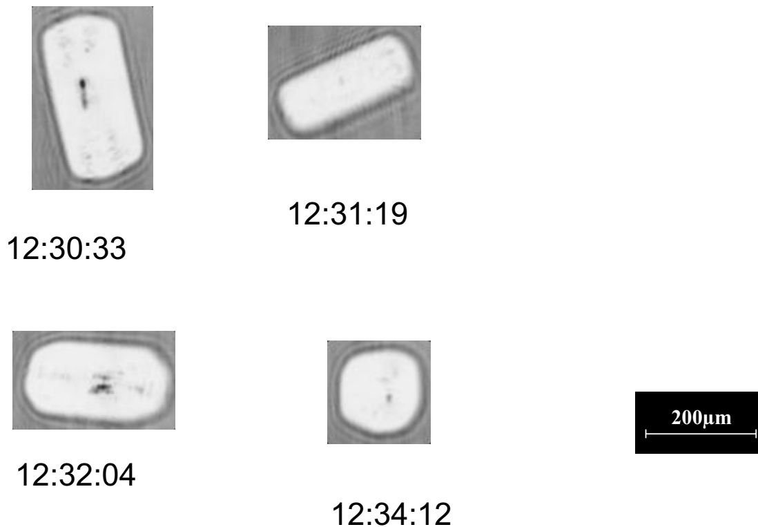
Fig. 6. Images of the four single ice crystals detected by the CPI in the thin cloud at about 3 km altitude.
