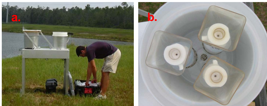
Fig. 2. Automated rainfall collector with a Plexiglas splash guard on the leading edge of the roof to avoid splash contamination during roof retraction (a) . Modified receiving bucket with three nested receiving bottles connected to polycarbonate funnels using PTFE-Teflon collars.
