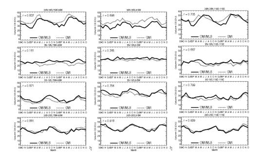
**Fig. A1.** Monthly time series comparisons of GMI (dotted curves) and OMI/MLS (solid curves) tropospheric column  $O_3$  (in DU) for three separate regions: American (left four panels), African (middle four panels), and Indonesian (right four panels).
