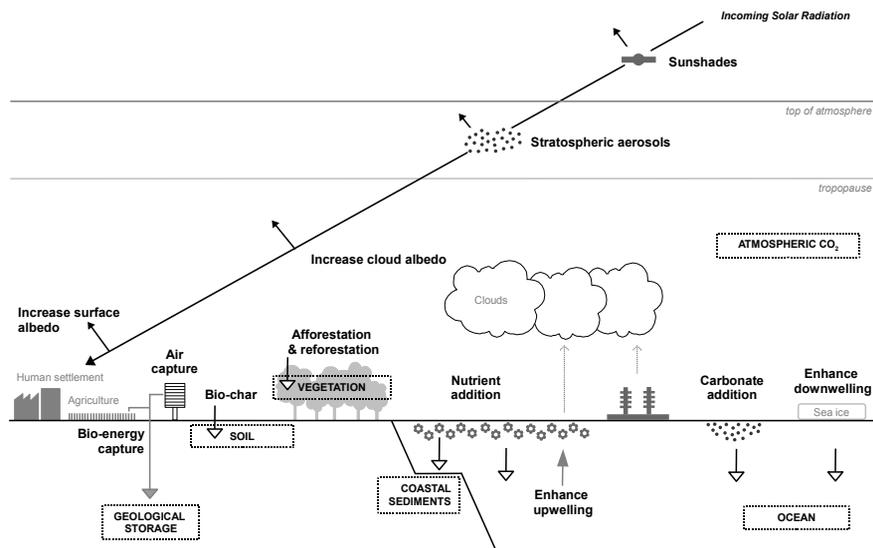
**Fig. 1.** Schematic overview of the climate geoengineering proposals considered. Black arrowheads indicate shortwave radiation, white arrowheads indicate enhancement of natural flows of carbon, grey downward arrow indicates engineered flow of carbon, grey upward arrow indicates engineered flow of water, dotted vertical arrows illustrate sources of cloud condensation nuclei, and dashed boxes indicate carbon stores. From Vaughan and Lenton (2009), not to scale.
