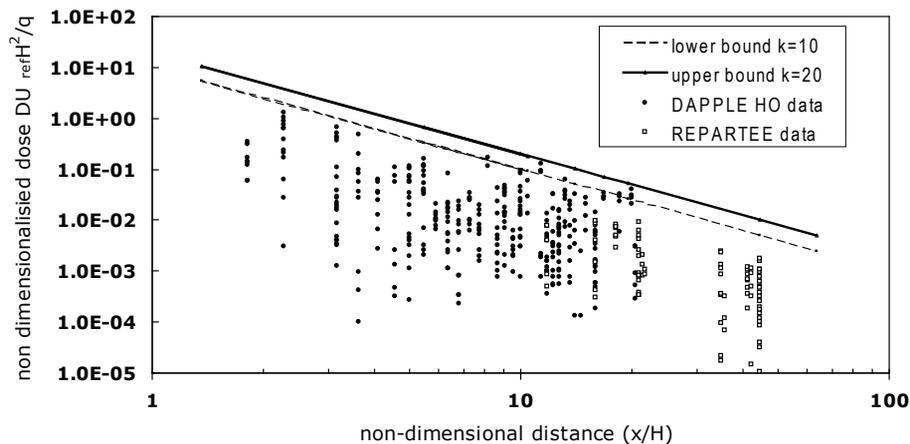
**Fig. 7.** Evaluation of simple correlation model based on experimental data from both REPAR-TEE and DAPPLE HO campaigns centred in London.
