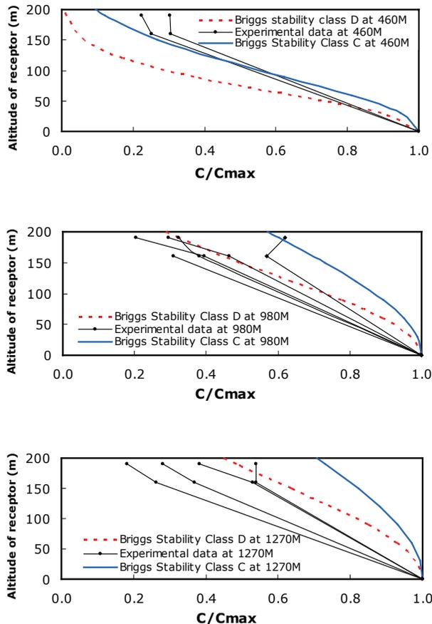
**Fig. 4.** Vertical gradient profiles for different source-receptor distances: 460, 980 m (2007 data); 1270 m (2006 data).
