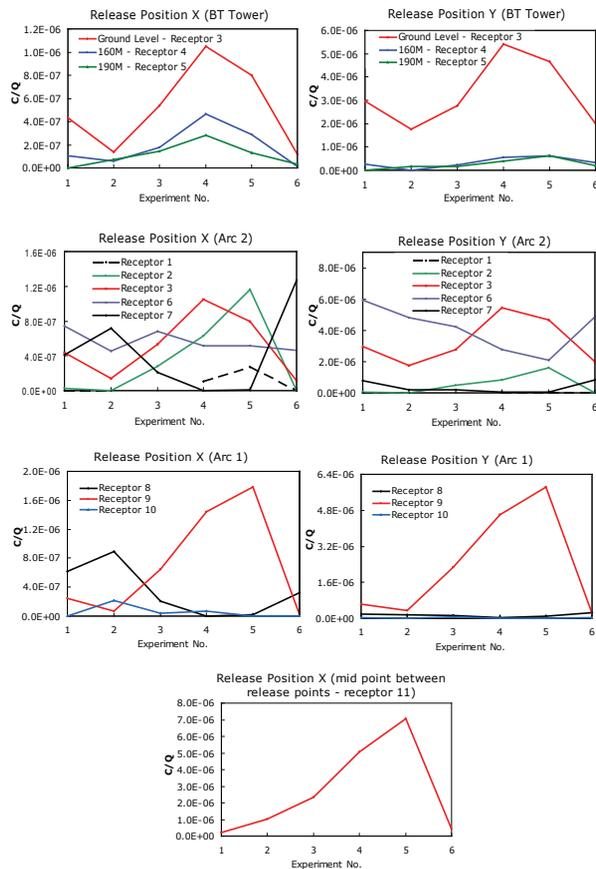
**Fig. 3.** Time-series of concentration for REPARTEE 2 (7 November 2007). Six experiments carried out: Release interval: 15 min, Sampling interval: 35 min, Starting concurrently at 13:00 with each experimental period lasting 45 min.
