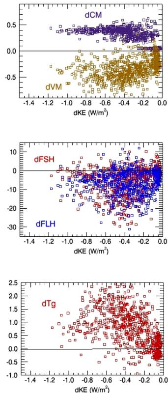
**Fig. 4.** Changes in surface momentum drag coefficient (dCM; unit-less), wind magnitude (dVM; m/s), sensible (dFSH;  $\text{W/m}^2$ ) and latent (dFLH;  $\text{W/m}^2$ ) heat fluxes, and surface air temperature (dTg; K) over the model grids where the kinetic energy losses (dKE;  $\text{W/m}^2$ ) due to wind turbines occur. Results shown are year 41–60 means of Run L minus Run REF.
