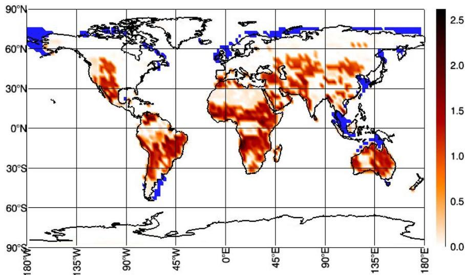
**Fig. 1.** Locations of land installations are indicated by the modeled change of surface drag coefficient (non-dimensional) averaged over the final 20 years of the 60-year Run L (see color code on right hand side). The drag values have been scaled by a factor of 1000. Also shown are the locations of offshore installation regions where the ocean depth is shallower than 200 m (blue shading).
