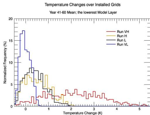
**Fig. 2.** Temperature changes (Run L minus reference, REF) in the lowest model layer resulting from large-scale deployment of wind turbines over land sufficient to generate 158EJ/year of electric power (upper panel); and normalized frequency of temperature changes over the installation regions in Runs VH, H, L, and VL (lower panel). Both refer to averages over years 41–60.
