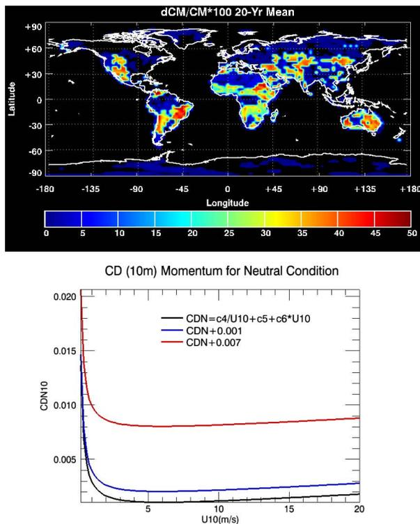
**Fig. 6.** Percentage changes of surface momentum drag coefficient ( $dCM/CM*100$ ) due to the simulated wind turbines over the land (upper panel); and surface momentum coefficients ( $CDN_{10}$ ) without (black line) and with (Run OL, blue line; Run OH, red line) the simulated wind turbines over the ocean (lower panel).
