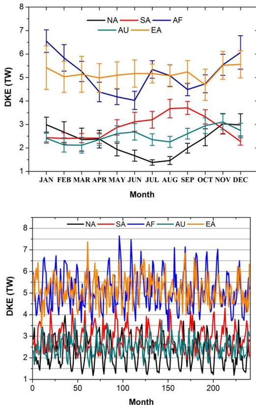
**Fig. 9.** Twenty-year (years 41–60) averages and standard deviations (upper panel), and all values (lower panel), of the monthly mean wind power consumption  $DKE=dKE/dt$ , Eq. (1) by simulated wind turbines installed in various continents: North America (NA), South America (SA), Africa and Middle East (AF), Australia (AU), and Eurasia (EA).
